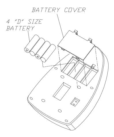
8. Insert 4 "D" size batteries into the back of the console.
